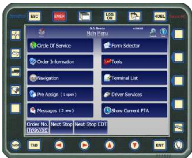
Figure 1. The main menu in XPE Truck provides access to information at a glance. All functions are available when the vehicle is stopped.
